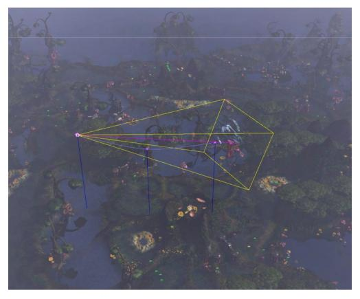
The camera is positioned and oriented in space. Via the CAMERA TAB, the designer can also set the field of view and clipping plane distances in order to control what is revealed to the player.
